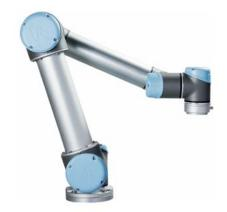
The robot can be programmed to move a tool, and communicate with other machines using electrical signals. It is an arm composed of extruded aluminum tubes and joints. Using our patented programming interface, PolyScope, it is easy to program the robot to move the tool along a desired trajectory.
