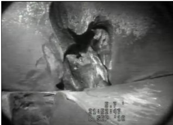
Figure 4.9.9. Erosion in the BOP.
